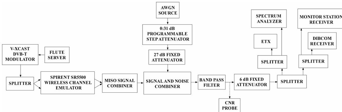
Fig. 2. Block diagram of laboratory test bench
