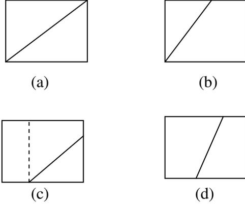
Figure 6. Surface subdivision scheme: (a) two 3 side patches; (b) one 3 and one 4 side patches; (c) two 4 side and one 3 side patches; (d) two 4 side patches
