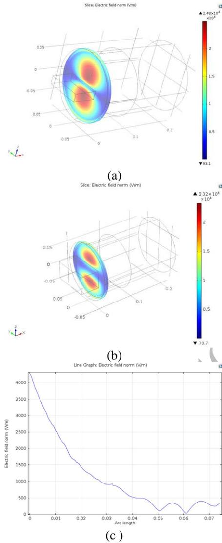
**Figure 7:** Electric field distribution with DPF
