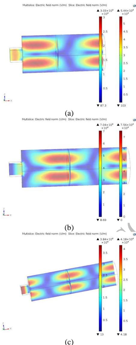
Fig. 8 Efield for various dimensions of the cavity
