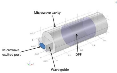
**Figure 5:** COMSOL geometry of the proposed microwave cavity
