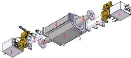
**Figure 1:** Existing microwave cavity with two magnetrons; (1) magnetron generators (magnetron source, measurements, and cooling), (2) stub tuners, (3) slotted waveguides, (4) microwave cavity and (5) air inlet/outlet
