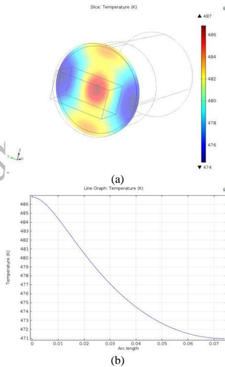
**Fig. 8:** Temperature profile of the DPF with WG2
