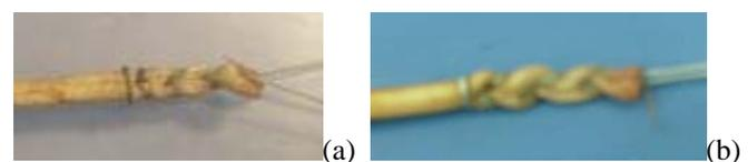
Fig. 1. The sutured region of a bovine digital flexor tendon before (a) and after (b) loading. The deformation of the tendon can be seen in the sutured area.
